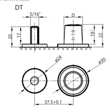
Terminal Torque Values in-Ib(Nm):17.69-26.53(2.0-3.0)
